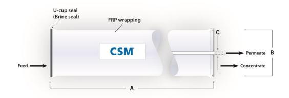
1. Each membrane element supplied with one brine seal, one interconnector (coupler) and four o-rings. 2. All RE8040 elements fit nominal 8.0 inch (201 mm) I.D. pressure vessels.
